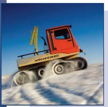
The structural steel frame and lightweight aluminum body, coupled with an optional accessory hydraulic pump, provides ample anchor points and hydraulic power to operate a diverse array of ancillary equipment.
